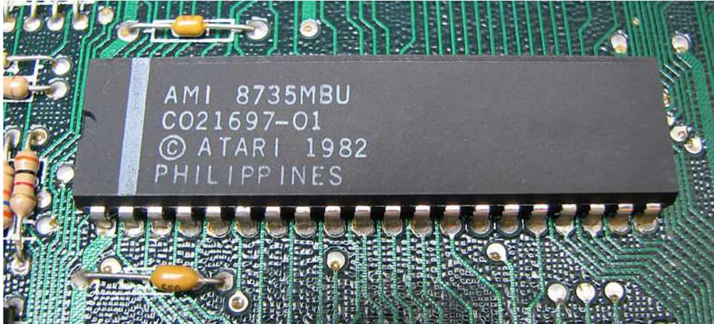
2. If ANTIC CHIP is socketed, remove it from socket and remove socket. If it is not socketed, You have to desolder it. After this operation, space after ANTIC CHIP should be clean from solder – like below. ANTIC CHIP will be needed later so do it carefully !
